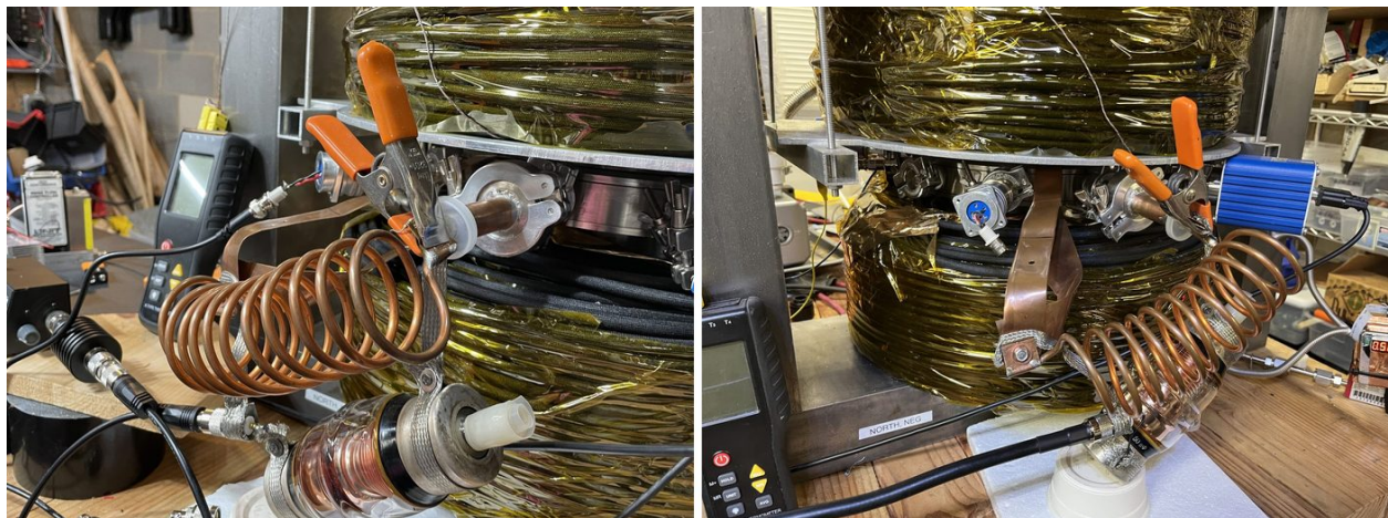
Figure 5. The matcher at port 6. Left, 2021-04-11: the bare copper tubing coil (the builder counts 11 turns) wound at the glass vacuum capacitor, whose concentric copper-cylinder electrodes show through the envelope at lower right; tinned braid runs to the copper ground strap, which disappears upward between the chamber lid and the pole; a spring clamp holds the strap to the feedthrough flange; the older UNIT mass-flow controller and the HT20 gaussmeter are in the background (media id: Live Photos/IMG_2658). Right, 2025-02-02, from the other side: the capacitor's label reads "50 nF" (50 pF, Russian surplus); the wide flat copper ground sheet runs from the feed-point braid up between the lower lid and the lower pole face; the LMR-400 feed enters at lower left on a styrofoam block; the four-pin filament/pickup feedthrough is at upper left, and "NORTH, NEG" is the pole-polarity label (media id: Live Photos/IMG_9642).
