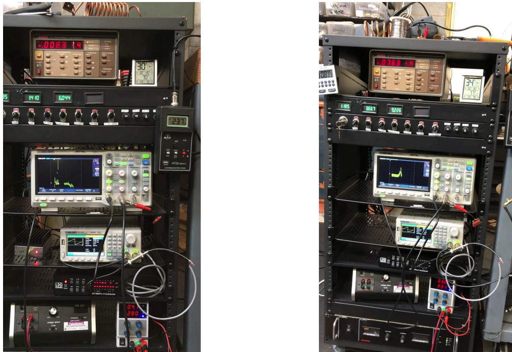
Figure 4 (left). Video frame, 2018-12-24, during a sweep. Top: Keithley 617 electrometer on its 10^{-9} A range. Right: HT20 gaussmeter reading 237 mT as the ramp passes through. Centre: Siglent oscilloscope in XY infinite persistence, the current-versus-field trace building from left; below it the function generator showing the triangle ramp. The three green panel meters are the vacuum-gauge readouts. First logged era, unbiased collector. Figure 5 (right). Video frame, 2020-05-31: a single clean peak on the persistence trace, electrometer reading -0.076 nA at the moment of the frame, countdown timer running. The log rows for this date carry no field value (the gaussmeter had failed on 05-25) and peak currents of 0.07–0.4 nA at 8.85 MHz; the trace shows the peak shape the numbers do not.
