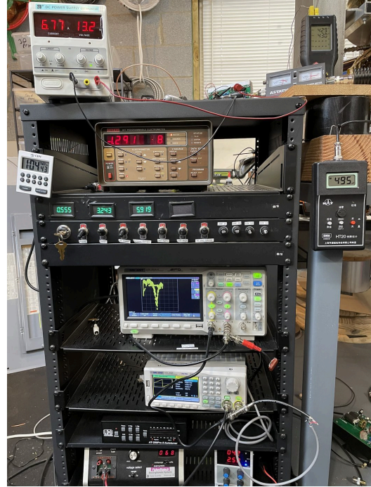
Figure 6 (left). 2021-03-06, the day the new RF amplifier went in: gaussmeter reading 623 mT near the top of the ramp, the resonance trace on the scope, electrometer in the 10^{-8} A range, timer at 1:04. The amplifier board and the Astatic SWR/power meter are on the bench at right, thermocouples at 42 °C. The log: "30W RF out, decent beam shape, 75C", -15 nA vs -5 nA at 587 mT / 8.981 MHz. Figure 7 (right). Same session, thirty seconds earlier: a twin-peak trace, gaussmeter reading 495 mT at the moment of the frame (the ramp is a triangle wave, so the instantaneous reading is not the peak field), electrometer -1.29 \times 10^{-8} A. Peak structure of this kind was noted throughout the diary but never recorded as data.
