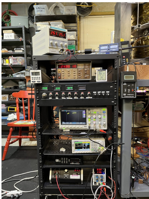
Figure 1 (left). The rack front on 2025-02-02, the last run. Top shelf: the RF final's DC supply (reading 2.51 A / 25.1 V), the Astatic PDC2 SWR/power meter and the thermocouple thermometer for the amplifier FETs. In the rack, top to bottom: Keithley 617 electrometer (reading in the 10^{-10} A range), the three green gauge meters (0.520 / 1.598 / 5.379 V), the keyswitch and toggle panel, the Siglent SDS1202X-E scope in XY mode, the Siglent SDG1032X generator, the LDG autotuner (still mounted, no longer in the RF chain), the FB 103 bias supply beside the small filament supply (2.35 A), and the Sorensen DCS 55-55 at the bottom. The HT20 gaussmeter hangs on the cart post at right. Figure 2 (right) . The control panel during the 2021-03-06 run. Gauge meters read 0.555 / 3.243 / 5.919 V (foreline \approx 0.025 torr; the middle gauge was noted as out of calibration in that day's log; high gauge 8 \times 10^{-5} torr N 2 -equivalent with hydrogen flow ing). Key in the keyswitch; toggles labelled Magnet · Power · RF Power · Vacuum Gauges · Diff Baffle · Diff Heat · Hi Vac Gauge; fused rail indicators 24 V 1 A · 28 V 3 A · 12 V 5 A · 15 V 1 A. HT20 at 495 mT; electrometer at -1.29 \times 10^{-8} A; run timer at 1:04:43; the resonance trace is on the scope below.
