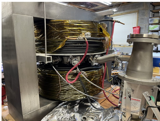
Figure 6 (left). Magnet, chamber and diffusion pump on 2024-08-03 (photographed while the machine was open to air between the 2023 and 2025 runs). The Edwards SI100 with its nameplate at right, the KF25 hose from its inlet-adaptor side port to the chamber, the ISO63 face blanked on top; the MKS 901P transducer on its chamber port; the coil ends with the welding-cable leads soldered on. Figure 7 (right) . Same day: the Harbor Freight 3 cfm roughing pump on its tray on the cart deck with the home-made exhaust filter (white cylinder) and the KF16 flex hose to the foreline tee; the orange knife switch in the magnet circuit is the never-used field-reversal switch, labelled with a warning about switching while the magnet is on; a 9 V battery string (bias supply) at lower right.
