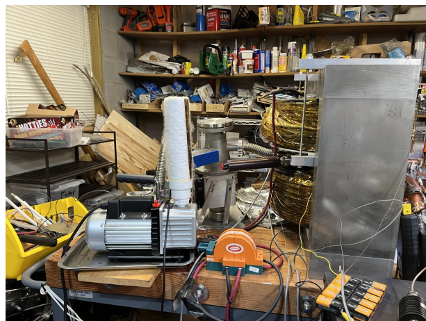
Figure 6 (left). Magnet, chamber and diffusion pump on 2024-08-03 (photographed while the machine was open to air between the 2023 and 2025 runs). The Edwards SI100 with its nameplate at right, the KF25 hose from its inlet-adaptor side port to the chamber, the ISO63 face blanked on top; the MKS 901P transducer on its chamber port; the coil ends with the welding-cable leads soldered on. Figure 7 (right) . Same day: the Harbor Freight 3 cfm roughing pump on its tray on the cart deck with the home-made exhaust filter (white cylinder) and the KF16 flex hose to the foreline tee; the orange knife switch in the magnet circuit is the never-used field-reversal switch, labelled with a warning about switching while the magnet is on; a 9 V battery string (bias supply) at lower right.
