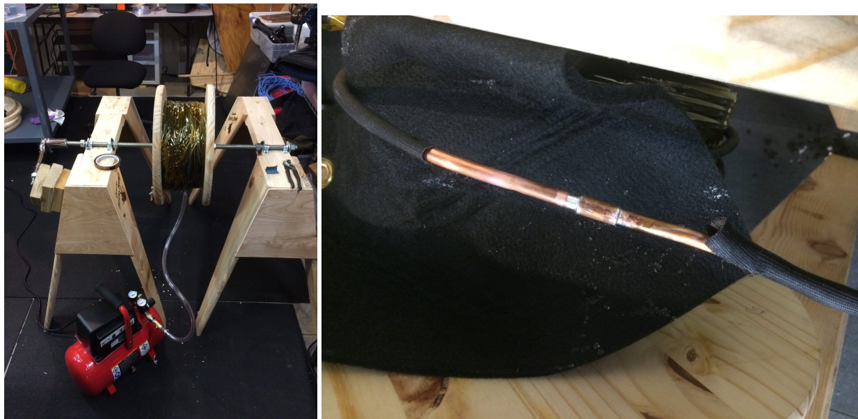
Figures 4 and 5, both 2017-05-28. Left: the winding stand — a partially wound coil on the plywood form between saw horses, the compressor at lower left connected by hose for the 100 psi pressure test, a roll of Kapton tape on the stand. Right: a completed joint — the 5/16 in coupler silver-soldered over the ends of two 1/4 in tubing sections, with the black fiberglass sleeving pulled back on both sides before it is slid over the joint.
