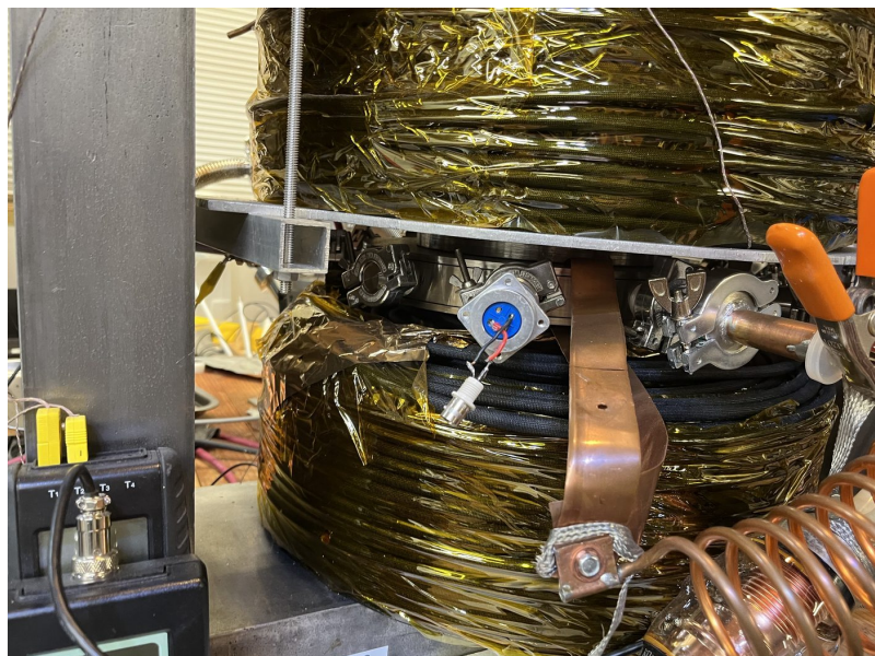
Figure 8. The magnet as it stands, 2024-08-03: the lower Kapton-wrapped coil, the chamber edge with KF16 flanges and a four-pin feedthrough in the gap above it, the copper RF ground strap, and at lower left the four-channel thermocouple meter (T1–T4) with yellow thermocouple plugs — the coil-temperature monitor that substitutes for cooling.
