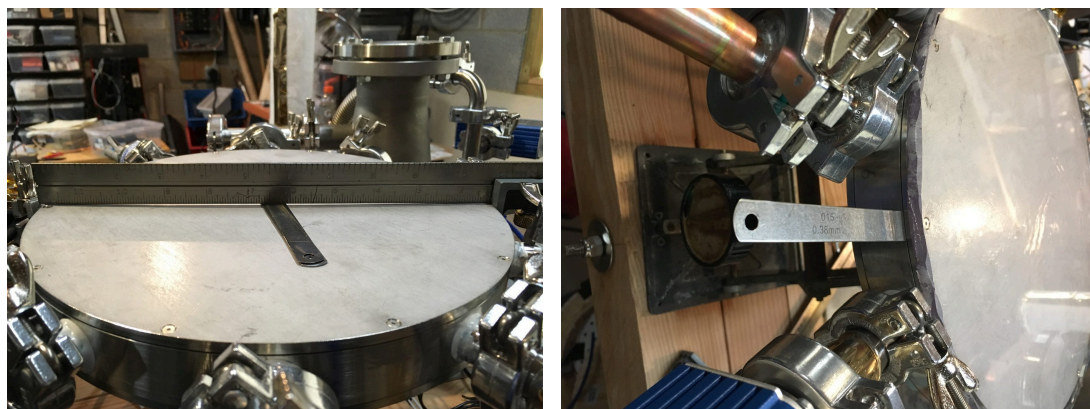
Figure 3. 2018-04-14, the deflection measurement. Left: the chamber on the bench under vacuum with a steel rule spanning the lid and a depth gauge at the center; behind it the SI100 with its ISO100 \rightarrow ISO63 adapter, KF25 side port and the flexible hose to the chamber. Right: a 0.015 in feeler gauge in the gap between lid edge and ring face at atmosphere; the gap grew to 0.016 in under vacuum. Port numbers ("6", "9") are scribed on the ring beside the flanges.
