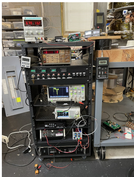
Figure 2. The instrument rack during a run on 2021-03-06 (media id IMG_2512). Top to bottom: a bench DC supply on the rack top, with the Astatic PDC2 SWR meter and a bare RF-amplifier board on the bench beside it; the Keithley 617; the DROK meter, keysw itch and rocker-sw itch panel; the Siglent SDS1202X-E with a resonance trace in XY persistence; the SDG1032X generator; the LDG AT-200PRO-II autotuner (still in the chain at this date) beside a Fisher electrophoresis supply; the Sorensen DCS 55-55 at the bottom. The HT20 gaussmeter on the bench post reads 623 mT; the CDN timer hangs at left.
