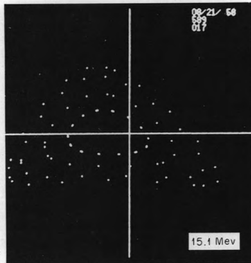
Fig. 31. Radial Phase Plots for Protons for Fields Obtained from Three-Sector Model Magnet.
